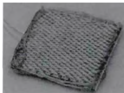
Figure 2. Soft electrodes made by steel fiber knitted fabric.
