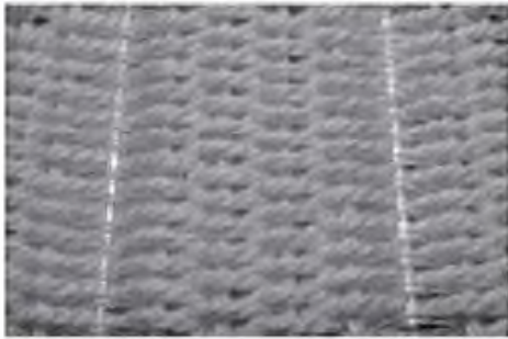
Figure 4. Textile sensor with optical fibers inductive sensor.
