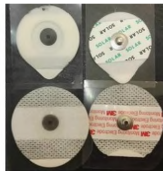
Figure 1. Ag/AgCl electrodes and its fabric composite electrode.
