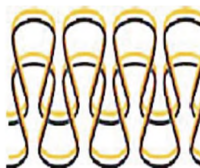
(a) Schematic diagram of knitting structure of fabric elongation sensor.
