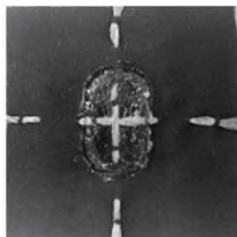
Figure 8. Embroidered fabric electrodes covered with silica gel.
