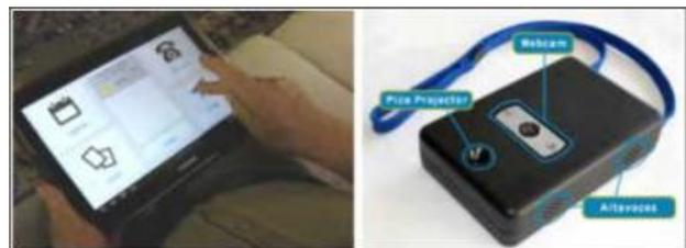
**Figure 3.** Interface devices: Tablet (left) and dcpair prototype (right).
