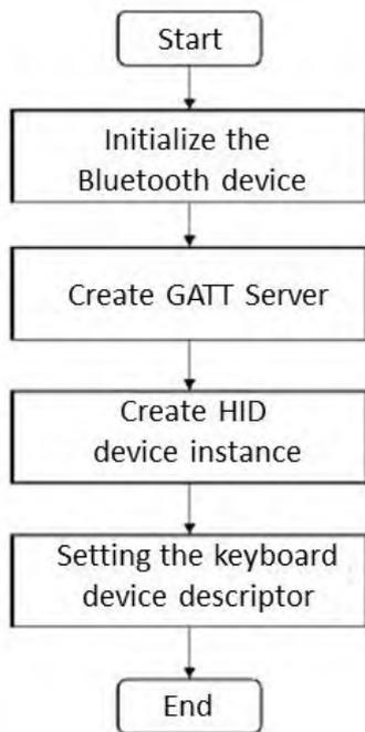
**Figure 6.** Bluetooth communication operation flow.
