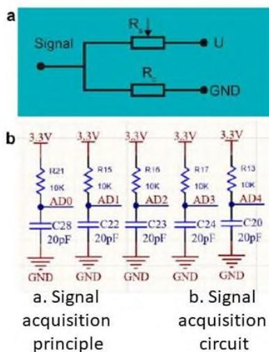
**Figure 4.** Signal acquisition principle and circuit diagram.
