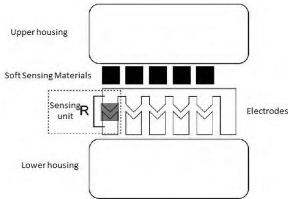
**Figure 2.** Sensor structure.
