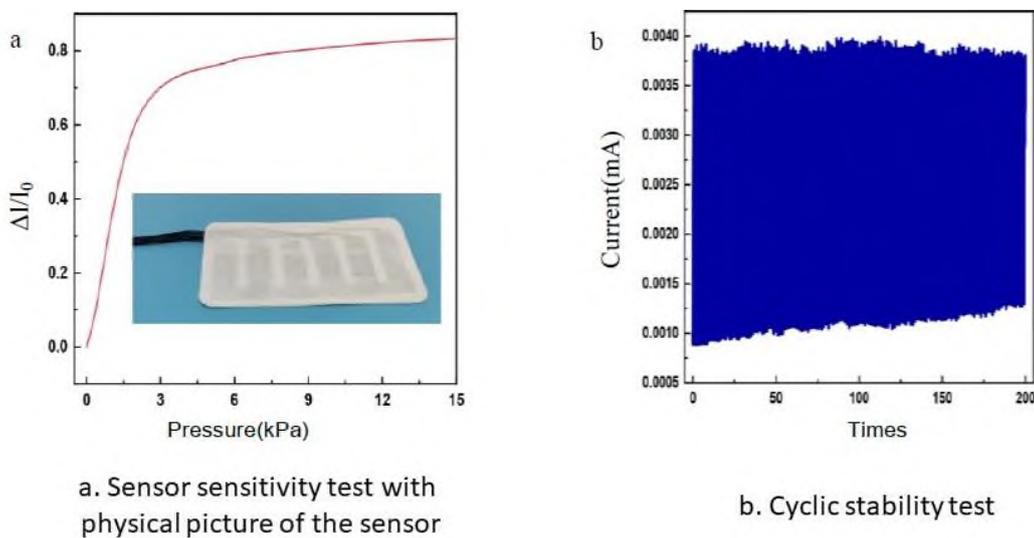
**Figure 3.** Physical and performance testing of sensors.
