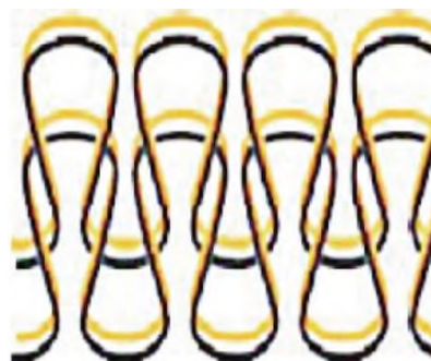
(a) Schematic diagram of knitting structure of fabric elongation sensor.
