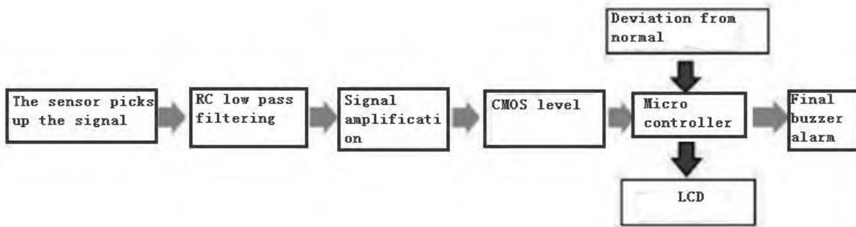
Figure 4. Structure diagram of the pulse monitoring module.
