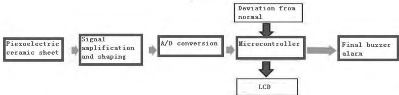
**Figure 3.** Structure diagram of the respiratory monitoring module.
