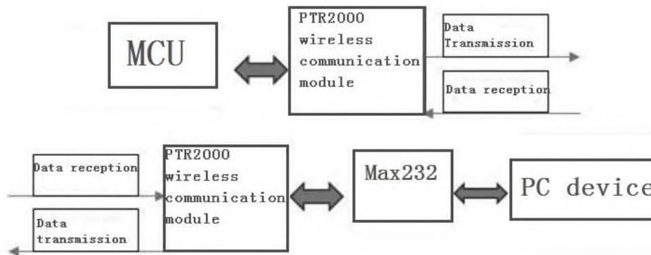
**Figure 8.** Working diagram of the infinite communication module.
