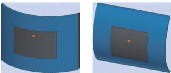
(a) Bending along antenna width (b) Bending along antenna length
