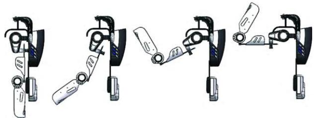
**Figure 6.** Motion simulation of flexion and extension in shoulder-elbow.
