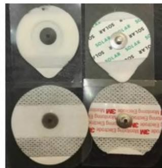
**Figure 1.** Ag/AgCl electrodes and its fabric composite electrode.
