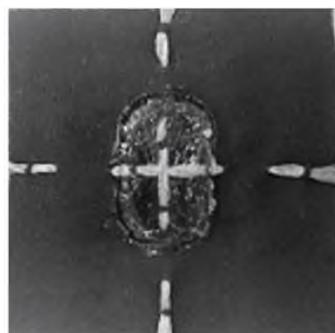
Figure 8. Embroidered fabric electrodes covered with silica gel.
