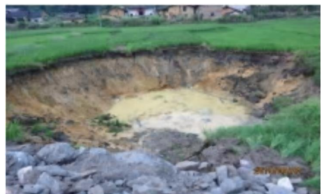
Figure 3 Surface collapse in muddy and watery areas.
