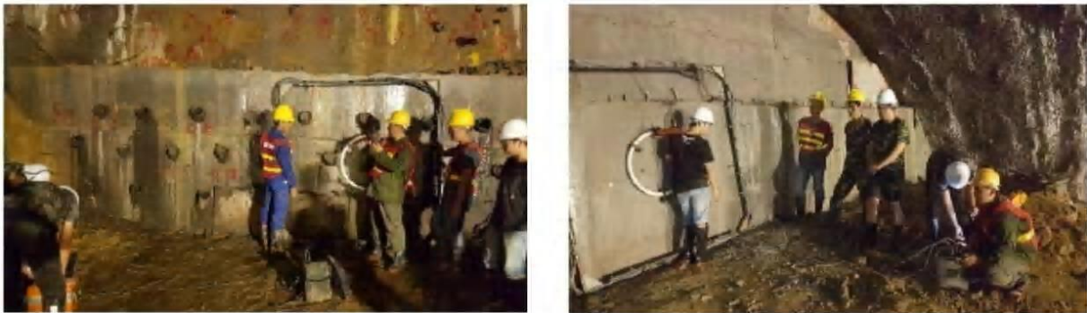
Figure 7 Transient electromagnetic detection of left and right holes.
