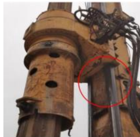
Figure 7 Sleeve drives the cylinder.
