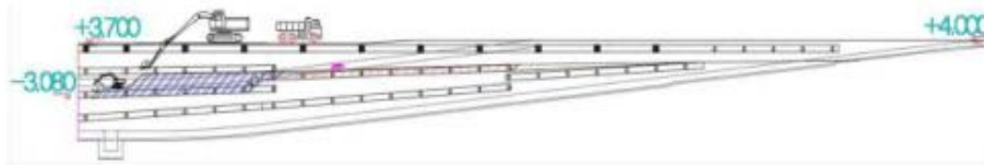
Figure 13 Schematic diagram of earthwork excavation on the first floor of underground passage four.
