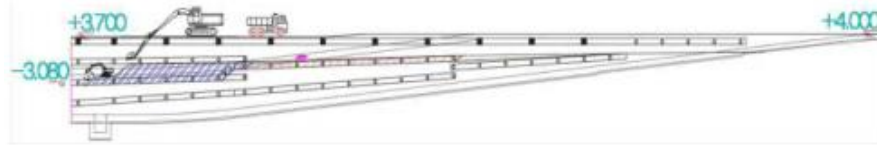
Figure 14 Schematic diagram of earthwork excavation for the second floor of underground passage four.
