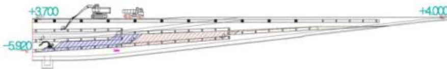
Figure 15 Schematic diagram of earthwork excavation for the third floor of underground passage four.
