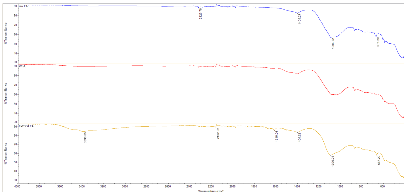
Figure 1. FT-IR spectra of RFA, WFA and Fe-WFA with a range of 4000–400 \text{cm}^{-1} .
