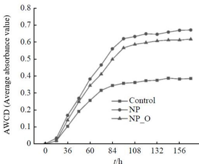
**Figure 2.** Variation in AWCD of petroleum contaminated soil under different treatments after 240 days.
