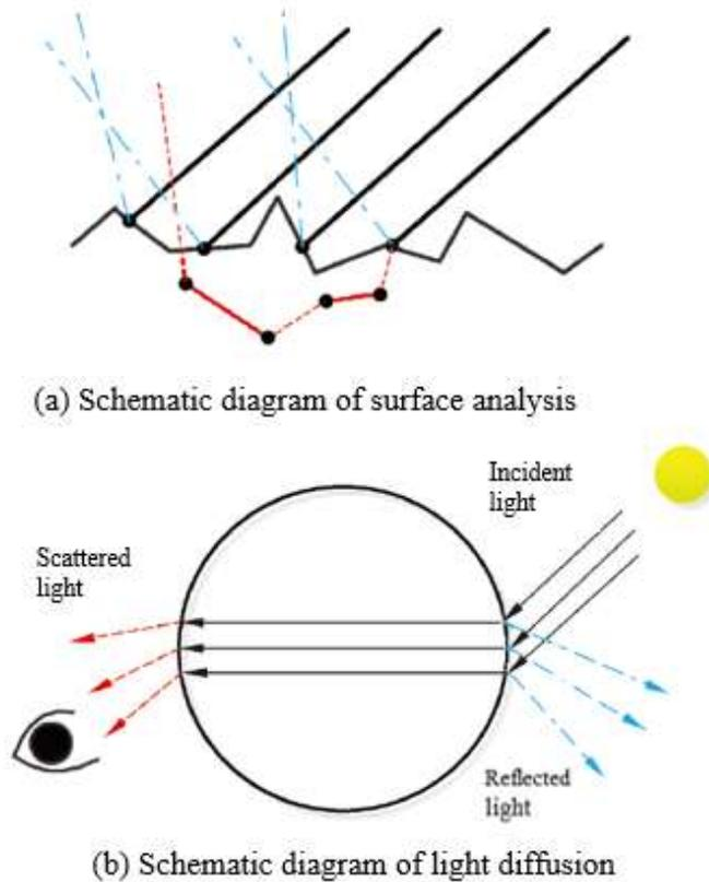
**Figure 1.** The scattering and reflection of light.
