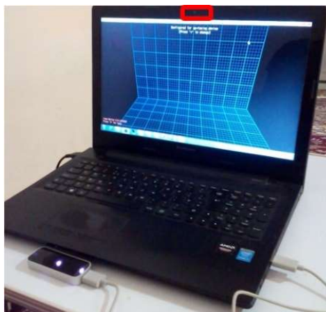
Figure 1. The positions of Leap Motion and the camera in the proposed interaction space. The camera is depicted in red color.
