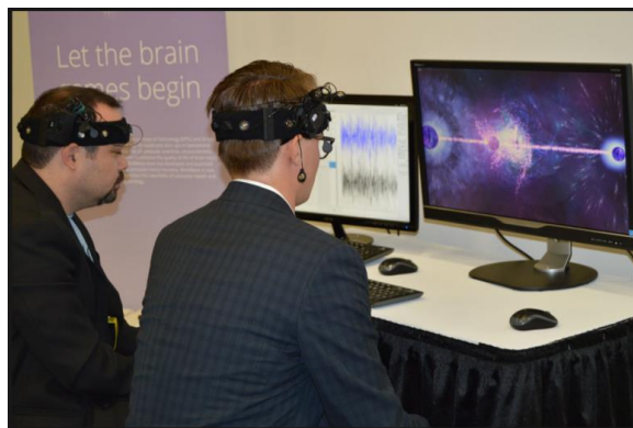
Figure 6. Controlling virtual reality activities through brain waves in the game, there is a stretchable magic ball on each side of the screen and a small ball in the center. The players' mental focus controls the magic balls, wearing headbands with sensors implanted on their foreheads. The game's objective is to use bursts of energy to expand the central ball and push back the opponent's magic ball. The larger the central ball expands, the stronger the player's mental power is demonstrated to be.
