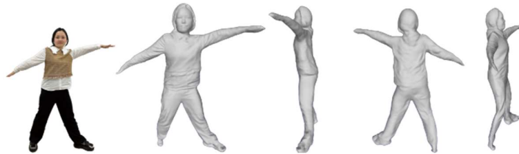
Figure 9. 3D human body reconstruction based on frequency domain completion method.
