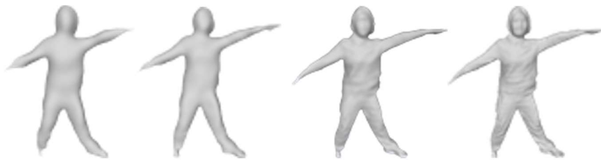
Figure 7. The reconstruction results of projecting the human body from the geometric space to the k (from left to right: k = 62, 250, 1000, 2000 ) dimensional frequency domain space based on the manifold harmonic basis.
