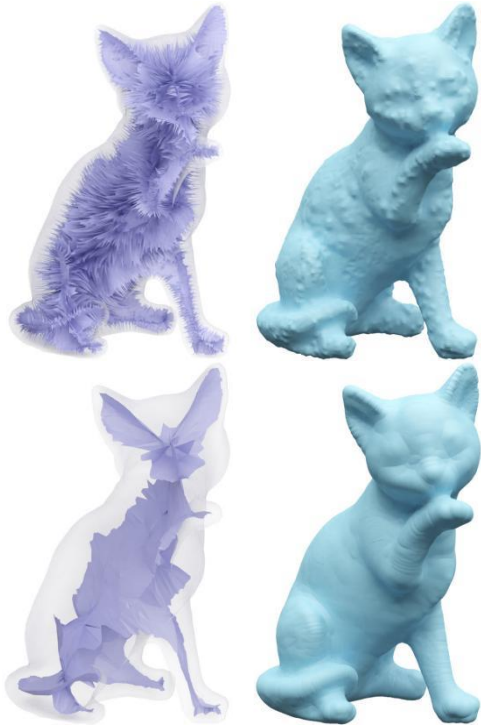
Figure 3. Comparison of “spikes” in medial axis transform. (top) Medial axis transform with lots of spikes (bottom) Simplified medial axis transform.
