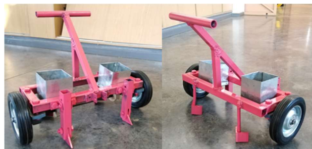
Figure 10. Constructed two-row single metering plate maize planter.
