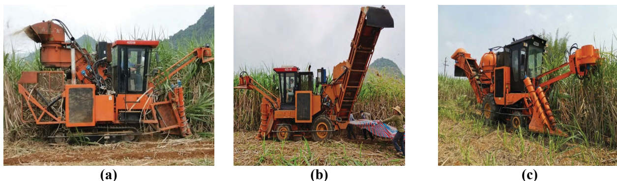
Figure 2. Field harvesting of sugarcane harvesters. (a) 4GQ-1c sugarcane harvester; (b) 4CZQ-180 sugarcane harvester; (c) 4GZQ-260 sugarcane harvester.
