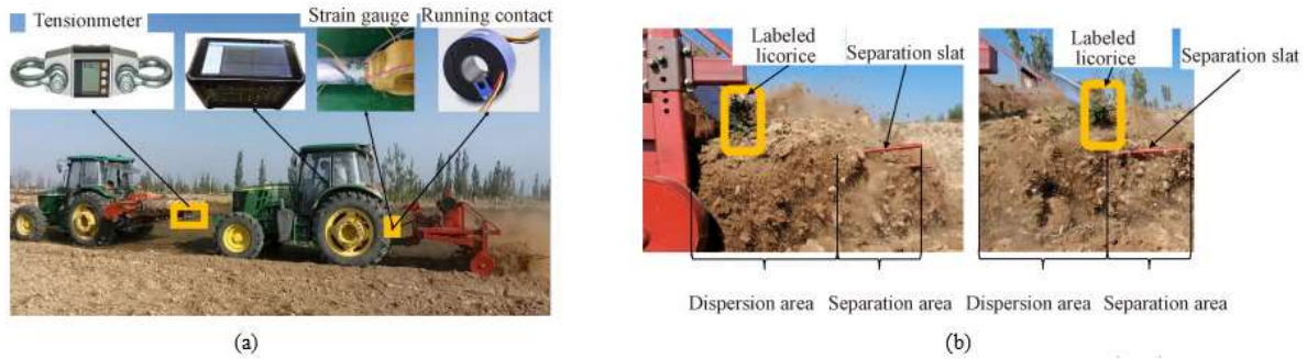
Figure 22. Field experiment of licorice harvest, (a). Experimental process; (b). Throwing effects of oscillating slat shovel.
