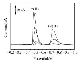
**Figure 2.** Anode stripping voltammograms of  $2.40 \times 10^{-7}$  mol/L Pb(II) and  $9.80 \times 10^{-7}$  mol/L Cd(II) at a: the bare GCE; b: Nafion/GCE; and c: Nafion/GQDs/GCE.
