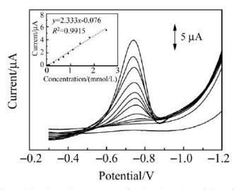
**Figure 6.** Differential pulse voltammogram for the detection of CAP from  $5.0 \times 10^{-7}$  mol/L to  $2.5 \times 10^{-3}$  mol/L at the Nafion/GQDs/GCE.
