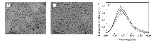
**Figure 1.** TEMI images of (**A**) low; and (**B**) high magnification of GQDs; (**C**) fluorescence spectra of GQDs (the excitation wavelength: a) 320 nm, b) 310 nm, c) 330 nm and (d) 340 nm).
