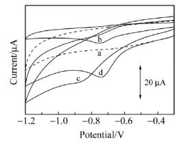
**Figure 4.** a: cyclic voltammograms of 0 mol/L and b:  $1.0 \times 10^{-4}$  mol/L CAP in TE buffer solution (pH = 7.0) at the bare GCE, c: Nafion/GCE; and (a, d): Nafion/GQDs/GCE.
