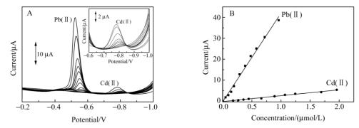
**Figure 3.** (**A**) different pulse voltammograms of Pb(I) and Cd(I) at the Nafion/GQDs/GCE; (**B**) linear plots of Pb(I) and Cd(I) striping currents vs. concentrations.
