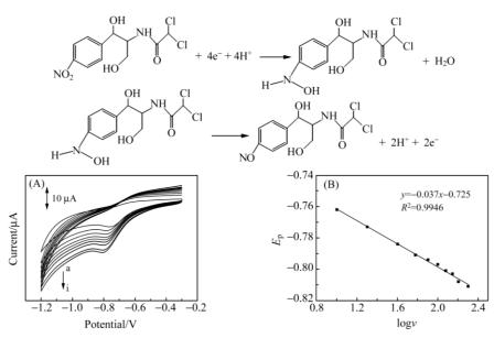
Figure 5. (A) cyclic voltammograms of  $1.0 \times 10^{-4}$  mol/L CAP at the Nafion/GQDs/GCE (scan rates (a $\rightarrow$ i): 10, 40, 60, 80, 100, 120, 140, 160, 200 mv/s); (B) linear plot of reduction potential vs. logv.
