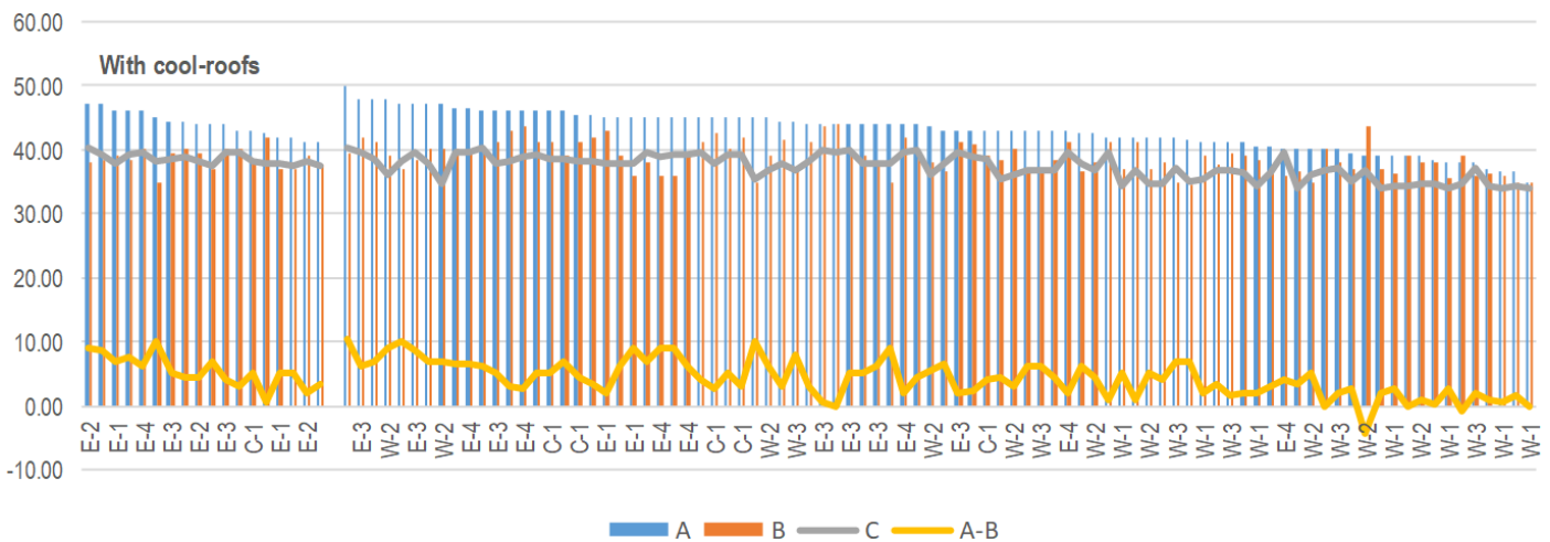
Figure 7. Temperatures outside and within DUs, city average and cool roof impact.
