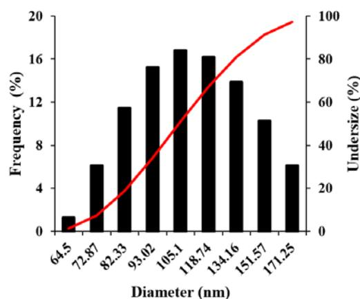
**Figure 3.** DLS results of the as-prepared MnO<sub>2</sub> nanozymes.
