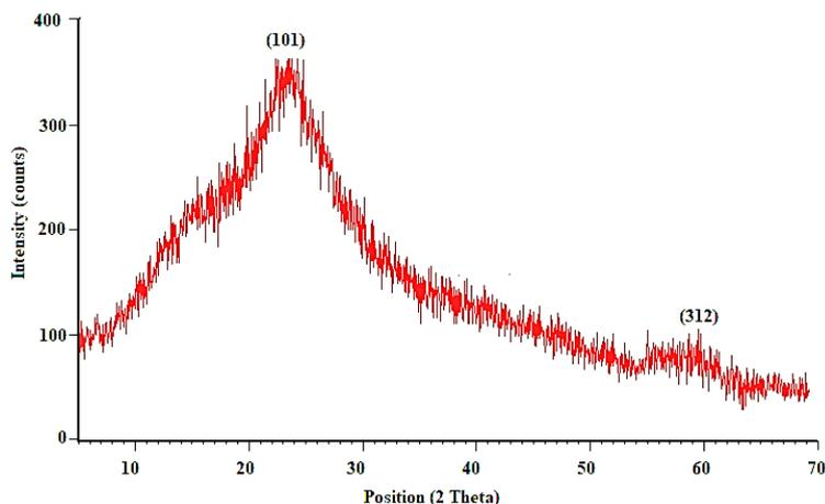
Figure 4. The XRD pattern of the as-prepared MnO<sub>2</sub> nanozymes.
