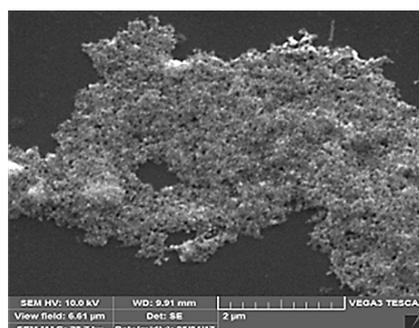
**Figure 1.** SEM image of the as-prepared MnO<sub>2</sub> nanozymes.
