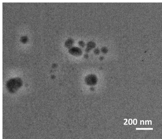
**Figure 2.** TEM images of the as-synthesized MnO<sub>2</sub> nanoparticles.
