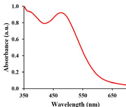
Figure 5. The UV-Visible spectrum of oxidation product of MnO<sub>2</sub> nanozymes-mediated oxidation of DAB.
