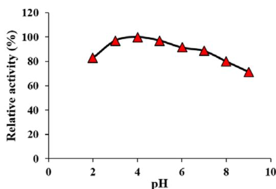
**Figure 6.** The pH stability of the as-prepared MnO<sub>2</sub> nanozymes.
