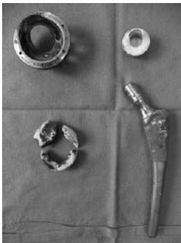
Fig. 3. The retrieved prosthetic components showed evident rupture of the acetabular liner and an elliptic deformation of the ceramic head.
