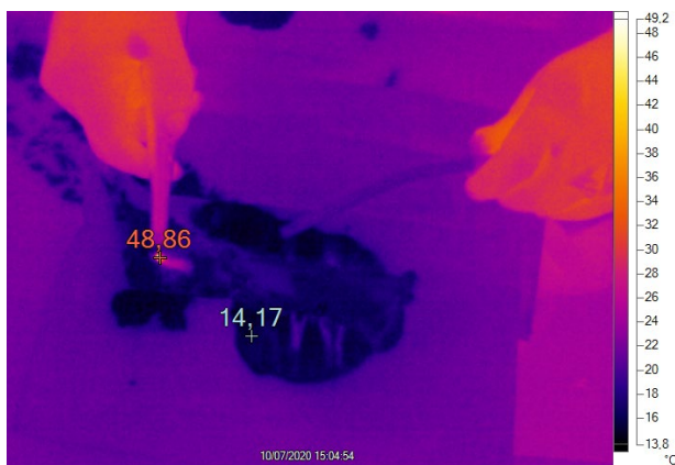
Fig. 5. Detection of anomalous rise in temperatures within hard tissue sample after Er:YAG incision without irrigation.
