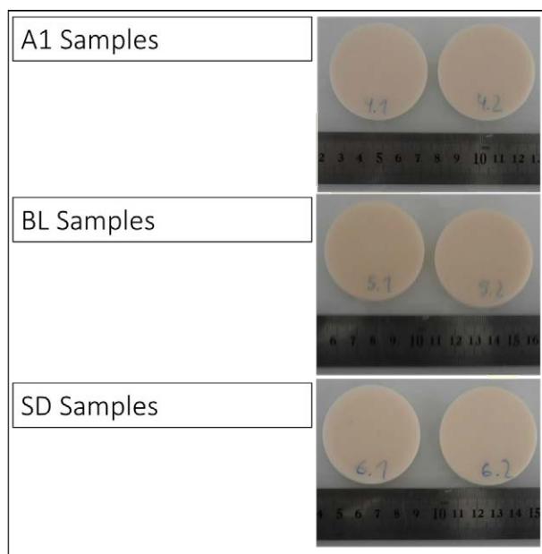
Fig. 2. Graphene-based PMMA (A1, BL and SD) unaged samples.
