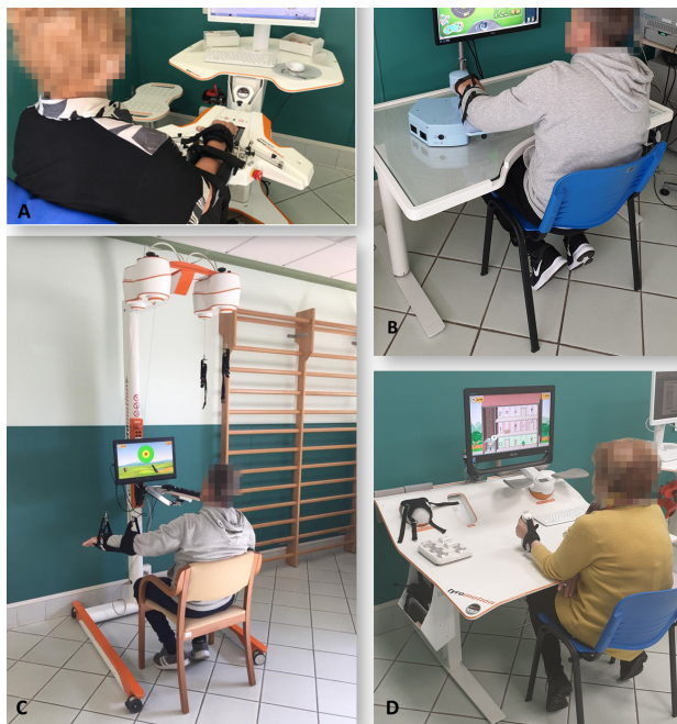
Fig. 1. Robotic and sensor-based devices used to treat the upper limb of patients assigned to the robotic group: (A) Amadeo (Tyromotion); (B) Motore (Humanware); (C) Diego (Tyromotion); and (D) Pablo (Tyromotion).
