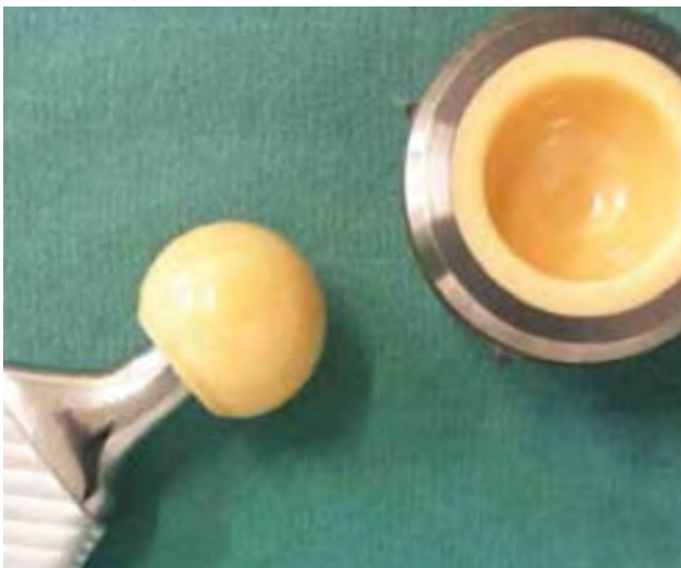
Fig. 1. Femoral head and liner in white Alumina and CoC bearing in Alumina-Zirconia.
