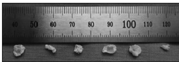
Fig. 2. The tissue constructs were cultured for 14 days. From left to right: TMJDCs (+), Co-culture (+), SMSCs (+), TMJDCs (-), Co-culture (-), SMSCs (-). Size shown in centimeters.
