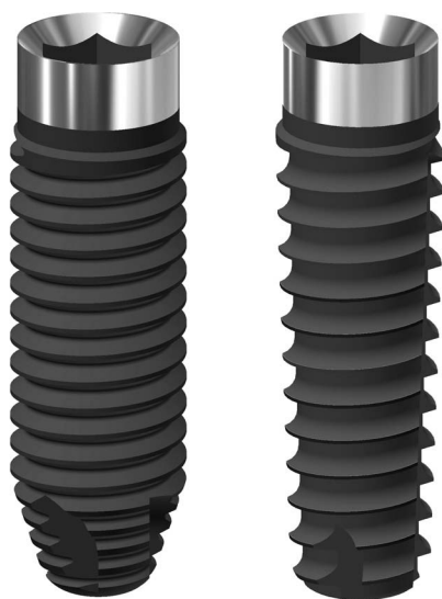
Fig. 1. The implant system considered for this study, had two different implant body configurations: one was cylindrical (on the left), while the other (on the right) was tapered. The two implant bodies differ for thread design (shape and pitch). Both the implants had a smooth neck (1.7 mm long). All the implant received the same surface treatment (i.e. sandblasting and acid etching).
