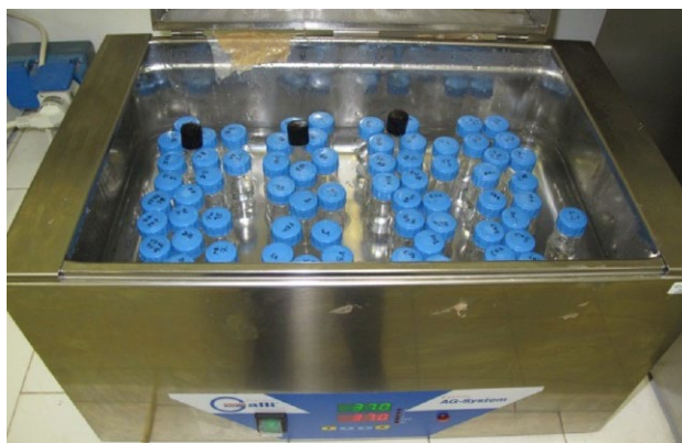
Fig. 2. The samples were immersed at 37 ° C for 30 days.
