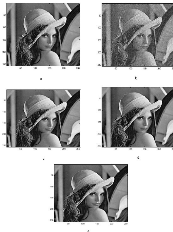
Figure 1. Denoising results of Lenna image, \sigma = 20 , (a) original image; (b) noisy image ( \sigma = 20 ); (c) translation invariant method; (d) top rule; (e) Wiener filter.
