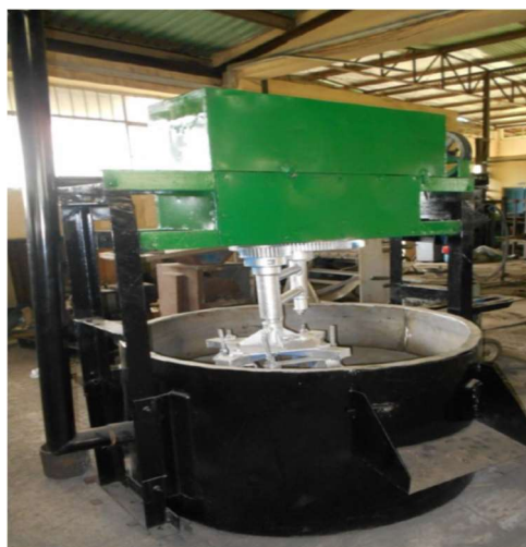
Figure 5. NCAM developed mechanical gari fryer.
