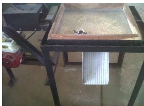
Figure 4. NCAM developed cassava sifter mass.
