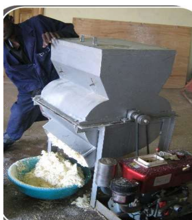
Figure 2. NCAM developed cassava grater.
