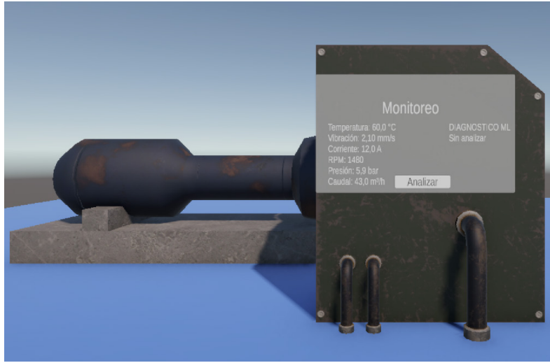
Figure 3. Initial digital representation of the industrial pump used for validating the embedded machine-learning diagnosis workflow. The in-scene panel displays the six operational variables used as model inputs (temperature, vibration, current, RPM, pressure and flow rate) and an idle “Diagnóstico ML: Sin analizar” status prior to inference, following the interaction pattern later reused, with asset-specific variables and models, throughout Stage 2.
